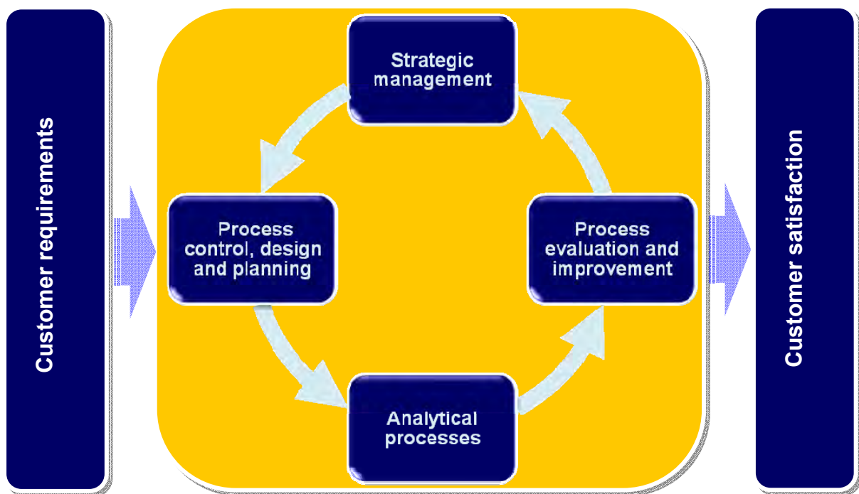
Figure 3. Overview of the ISO 22870:2016 process-based quality management system framework. The framework consists of four major stages: 'strategic management'; 'process control, design and planning'; 'process evaluation and improvement'; and 'analytical processes'. Each stage contains specific subclauses of ISO 22870:2016.
